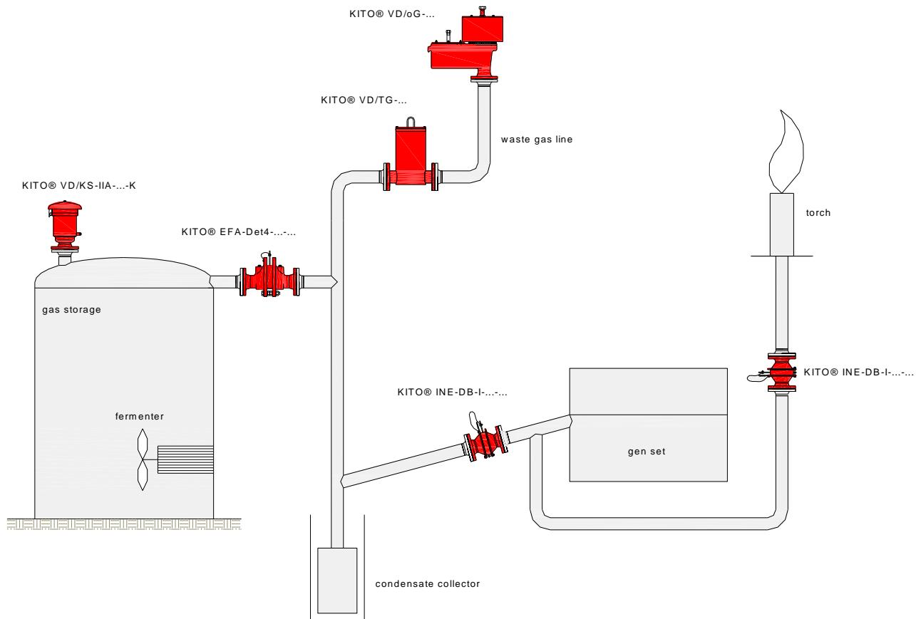
Bi-directional in-line detonation flame arrester, short-time burning proof KITO® EFA-Det4-IIA-.../...-1,2 (G 22 N)
